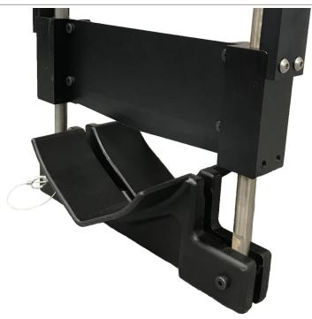
While wearing gloves, remove rubber guard before cutting pipe.
