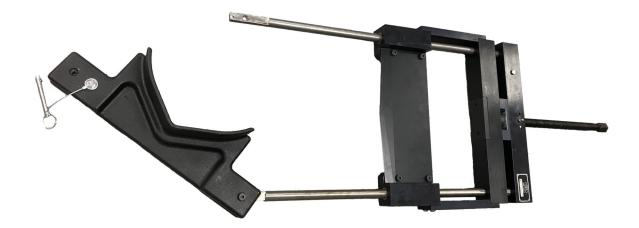
Turn handle and open blade all the way. Pull pin to allow bottom of V-Base to swing out. Place cutter over pipe. Swing V-Base back and replace pin.
