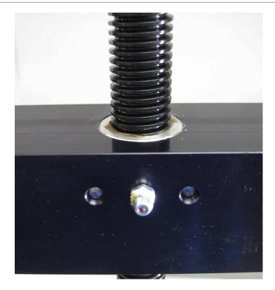
Make sure feed screw is kept greased and free of dirt. If dirty, wipe clean and reapply grease per instructions below.
